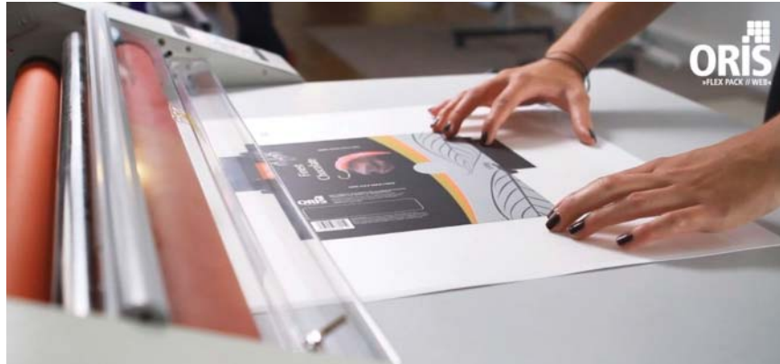
Figure 11 – Lamination to any press stock for realistic prototyping and proofing
