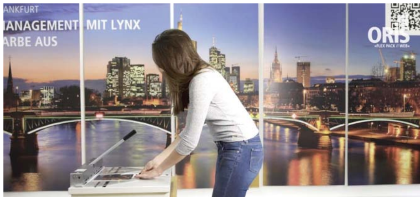
Figure 12 – Registration to 0.10 mm accuracy device to device using CGS Punch System
