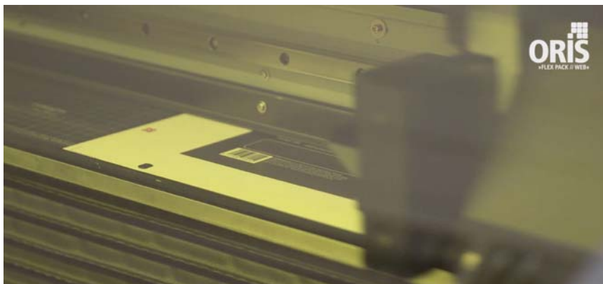
Figure 16 – Printing the foiling separation on the Roland LEF in order to apply the varnish adhesive for foiling
