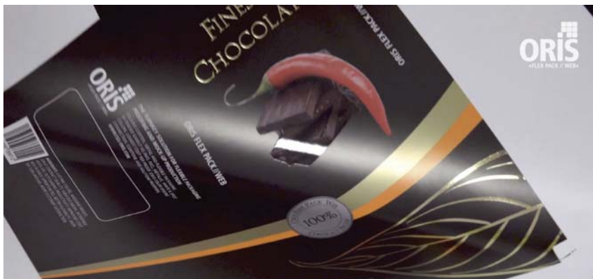
Figure 22 – Additional finishing effects are possible by returning the proof to the LEF-300 to add spot varnishes
