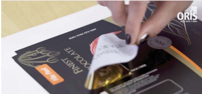
Figure 20 – Removing excess foil
