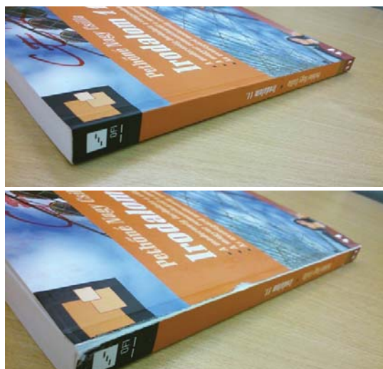
Figure 4: A/4 format, No.25-27 thread-stitched school book with a considerable extent of spine edge abrasion
