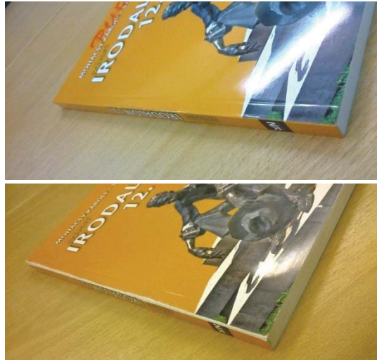
Figure 3: The largest extent of spine edge abrasion has been experienced for B/5 sized book No.10-12 In the A/4 format, the best final result has been achieved by the 410-gram, thread-stitched school book (Figure 4). Its cover is of 260 g/m 2 weight. During the test, abrasion apparently occurred after the 50th minute, but it did not change drastically even by the end of the 60 th minute.
