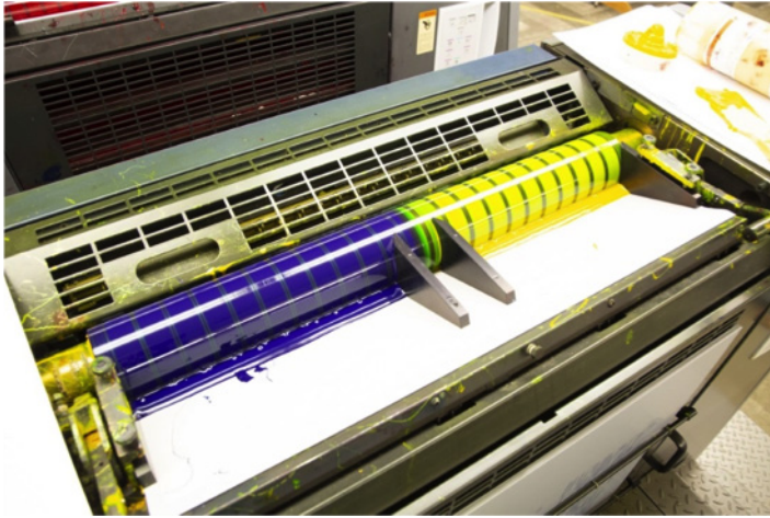
Figure 6. The ink tray shows no mixing after oscillators are disengaged
