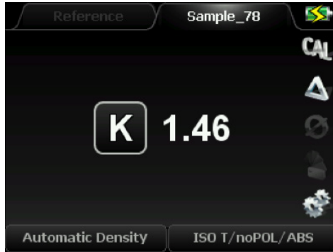
Figure 3. Visual reflection density of a black specimen recorded by TECHKON SpectroDens device
