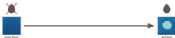
Fig 1. Hydrochromic ink (irreversible) changes its color from blue to transparent
