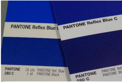
Figure 6: in the past different series of Pantone Color Guides could show rather big differences (picture from 2012)
