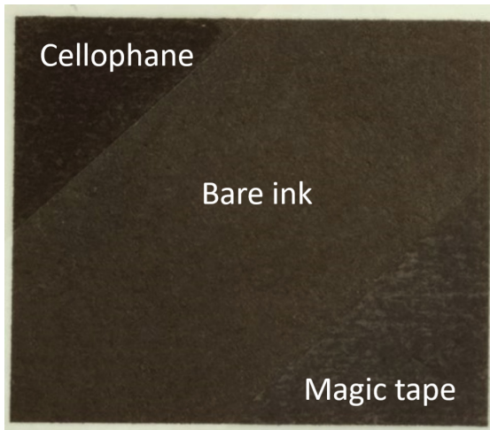
Figure 2 – The effect of tape on ink on uncoated paper
