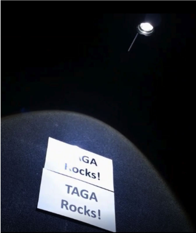
Figure 7 – Light reflecting at or near the specular angle
