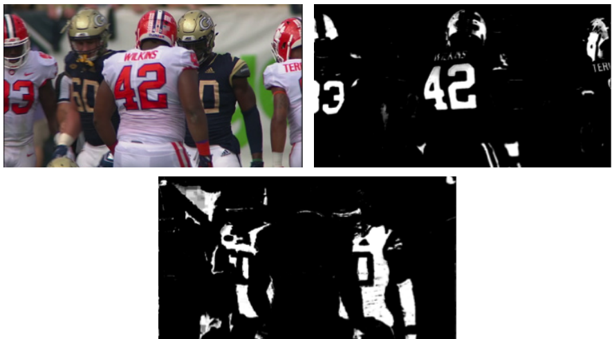
Figure 3: Segmentation masks for selecting Clemson orange (bottom left) and Georgia Tech navy blue (bottom right)
