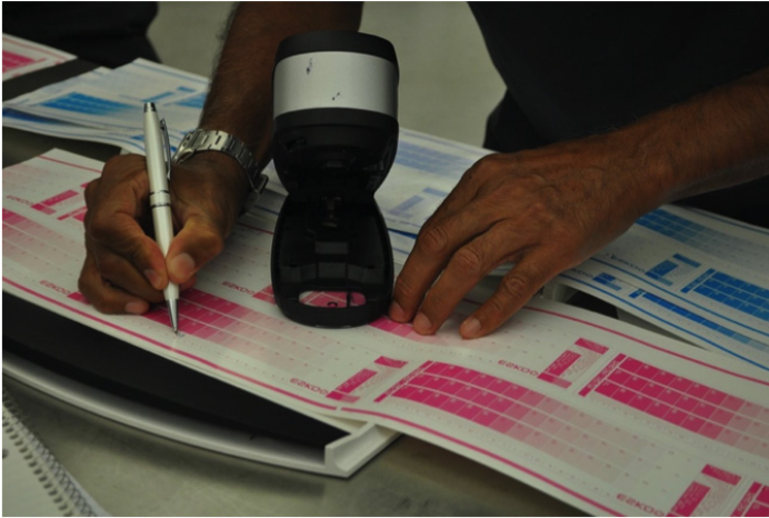
Figure 2: Press form used for the optimization run
