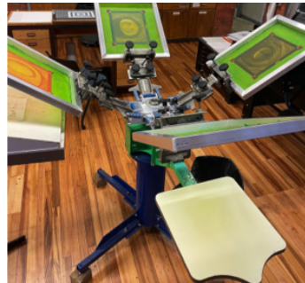
Figure 17: Registration and set up proved to be time consuming even with the color-coded screens. The yellow mesh decreased the visibility of the yellow color separation.
