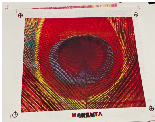
Figure 18: Four-color peacock feather sample produced. This CTS system was capable of imaging the screens to print CMYK product, however the quality of the final product needs improving. The color gamut produced did not match the color gamut requested.
