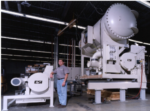
Fig 2. The New low voltage EB unit addressed the size issue of the older 150-200 kV EB unit
