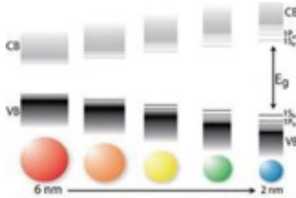
Figure 3. Gap evolution between QD of decreasing sizes. Source : Chem. Soc. Rev., 2011
