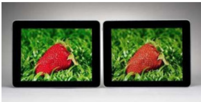
Figure 6. Comparison of a screen containing QDs ( on the left) and without (on the right). Source: American Chemical Society, 2014
