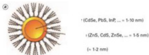
Figure 5. Schematic structure of a fluorescent semiconductor colloidal heart-shell nano-crystal.
