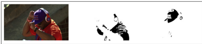
Figure 2. Segmentation masks for selecting Clemson orange (middle) and Clemson purple (right) from the original video frame (left).
