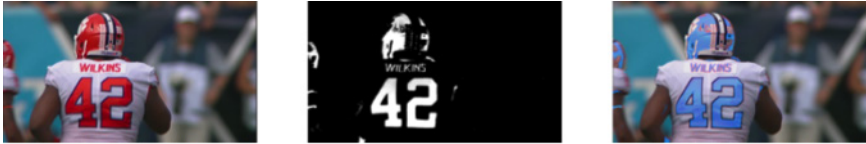
Figure 3. A grayscale mask (middle) can be used to shift the color of target pixels of an original frame (left), creating an augmented image (right). In this example, Clemson orange is changed to the University of North Carolina's blue.
