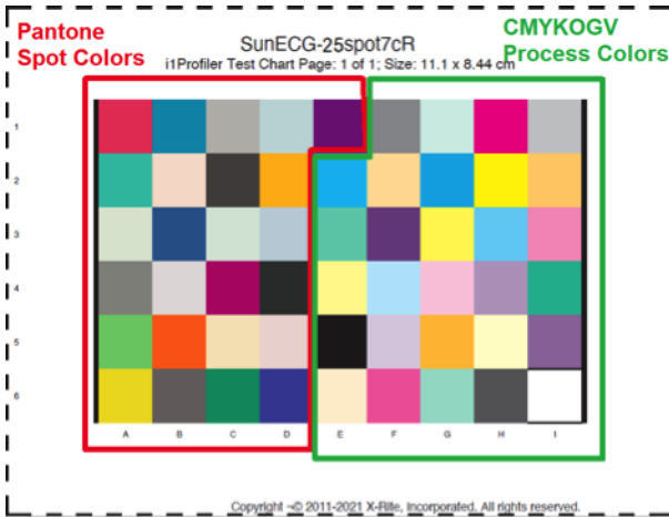
Figure 3: The colors in figure 2 are randomized and put into a test chart format suitable for i1iO. The chart was then placed into the press form layout.
