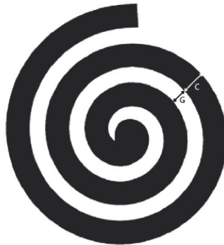
Figure 9: SPIR@L screening has 2 extra parameters on top of the standard AM parameters. The thickness of the spiral (Curve) and the size of the white space between 2 revolutions (Groove)
