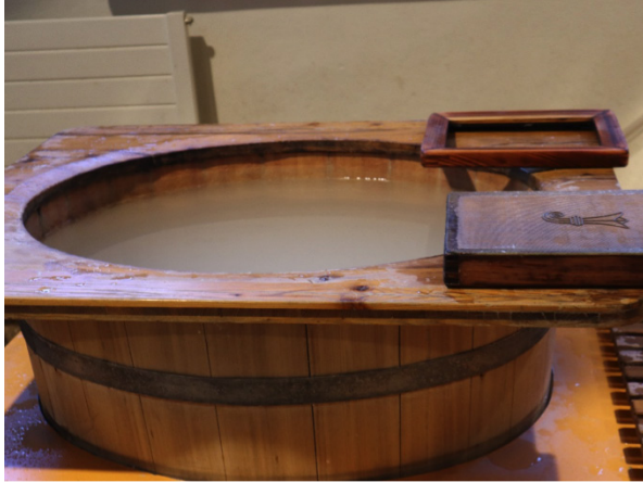
Figure 3: Vat with mold and its frame on the right side of the vat
