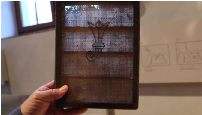
Figure 4: Close up on the mold with horizontal wooden ribs and Basel's blazon as watermark.
