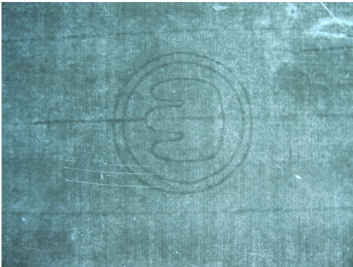
Figure 10: Beta-radiography of the watermark under investigation
