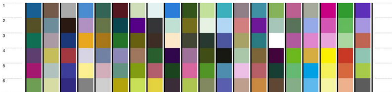
Figure 17. Final target for smooth surface papers, with 120 patches, in all quadrants, with neutrals and with 24 colors from the Xrite Colorchecker
