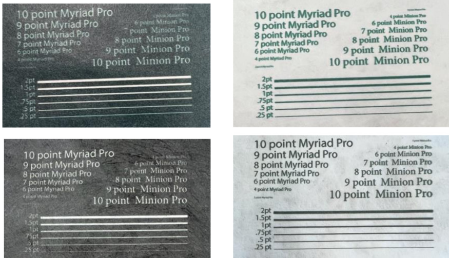
Figure 14 Positive and reversed text and lines printed by UV inkjet (top) and Latex (bottom) over rich black (left) and in PMS 3435 (right)
