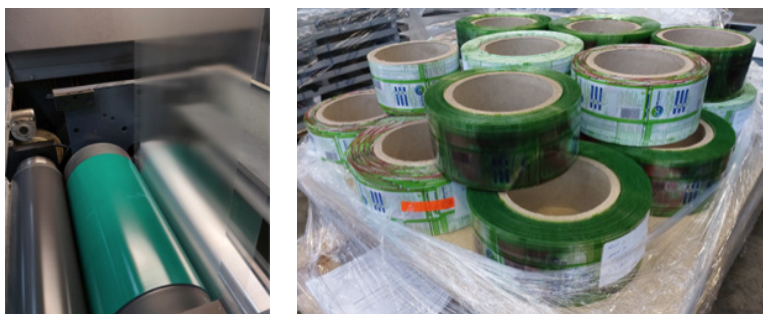
Fig.5 Left: Application of water-based deinking primer on an in-line flexo coater. Right: Slit and sleeved reels ready for deinking testing.
