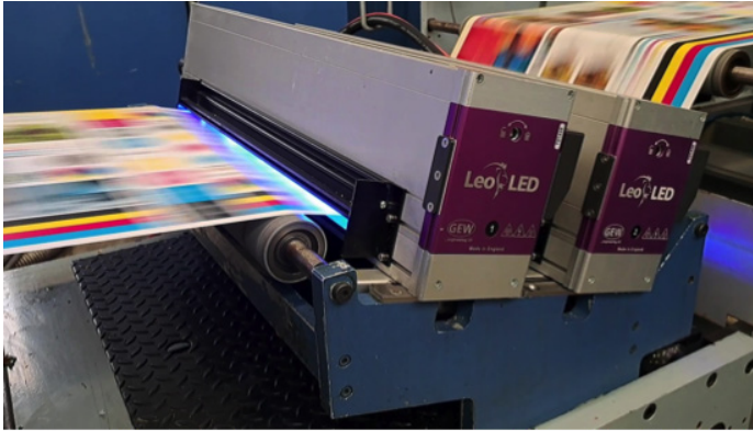
Fig.10 Integration of two LED-UV lamps from GEW as end-curing test system on a web-offset press, model Vision
