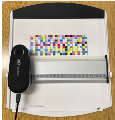
Figure 2: Offline measurement using the EFI ES-2000 spectrophotometer
