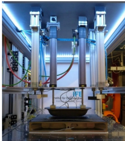
Figure 1. Forming tool “double dome” at IFB
