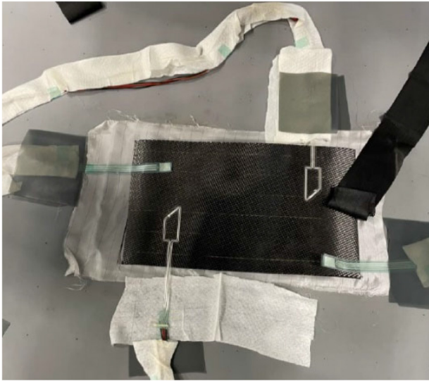
Figure 14. Two printed strain sensors attached to the carbon fiber mat prepared for the forming process The low-cost sensor performed so well that the project partners IFB (application), Balluff GmbH (electronics and system environment) and HdM (printing) decided to apply for a patent. Currently the patent is pending.
