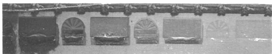
Figure 3 Ink-Colored Blanket Piling. Upper photo shows example of black (previous-down ink) colored piling of nonimage area of yellow blanket. Piling appears as raised deposits of ink. Lower photo shows similar piling in star target areas on same blanket; from left to right, colors are black, black, cyan, cyan, magenta, magenta, yellow and yellow. Severity of piling corresponds to color sequence of black, cyan, magenta, and yellow in that black piling is the heaviest and yellow is the lightest.
