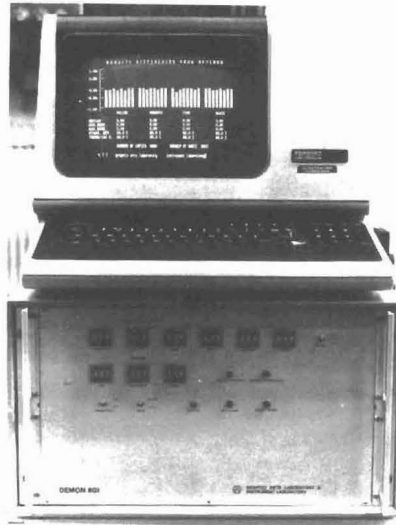
Figure 3. The display and the control panel of the web densitometer
