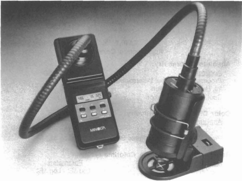
Figure 1. An inexpensive, portable filter colorimeter.
