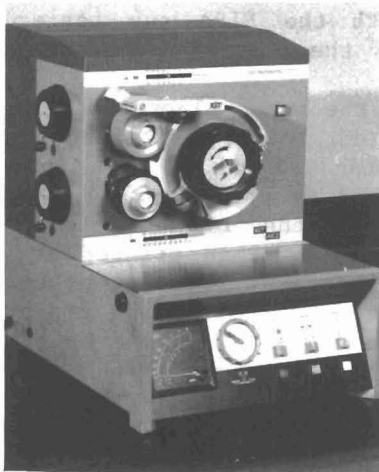
Figure 20. The IGT printability tester [99] set up for a wet-pick test. The film of water is applied to the paper at constant speed with the upper rubber roller. The pick test is then performed in the accelerated mode.
