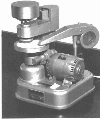
Figure 5. The Pira rub tester is used in Meret's dust test [4] and in the Elphick test [102] to rub the prints from the GFL printing unit [100].
