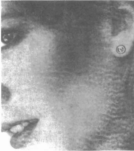
Figure 1. The wavy appearance of the print is caused by the accumulation of fine lint on a newspaper offset blanket [99]. Flexing of the blanket causes the lint to move in waves across the blanket.
