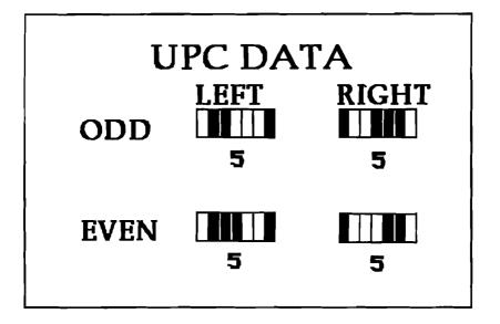
The form of the symbol includes a number system character, a five digit manufacturer's identification number, a five digit item identification and a check digit. Under certain conditions, the data can be compressed to six digits (Version E), reducing the real estate required by the symbol. Outside of the United States, an additional digit is used to encode the country of origin.
