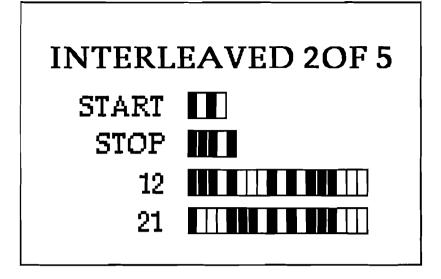
Each character consists of five elements, the two wide elements representing binary ones and the narrow elements representing binary zeroes. Only numeric data can be encoded.
