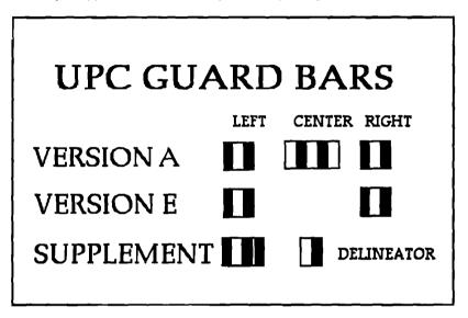
UPC characters are encoded continuously. Each character is made up of seven (7) modules which are divided into two bar and two space elements. Each element can be from one to four modules wide. Each character can be composed four ways depending on its position on the right or left side of a symbol or the character may be odd or even parity, if the application requires. Fortunately, computerized film master generators are used to produce symbols according to specifications.
