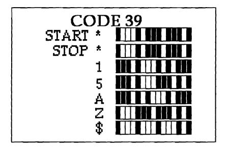
Tests of actual samples of Code 39 bar codes have resulted in substitution error rates of less than one error for each million or more characters scanned. Fair quality printing, resulting in one substitution error for each one million characters scanned, is expected to produce a first read rate greater than 90%.
