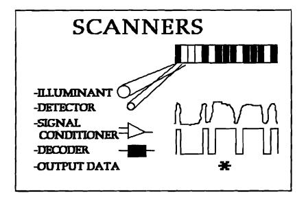
Fixed industrial scanners generally move the beam in one direction and wait for the label to move past the scanner. Some of these scanners do not move the beam at all, but depend upon movement of the label for scanning.
