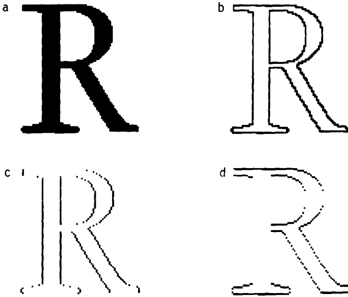
Fig. 4 Outline Points Associated with Various Scanning Systems. a. The letter R, on a 128x128 grid. b. Computer-generated closed outline with contiguous points. c. Outline points for horizontal scanning. d. Outline points for vertical scanning.
