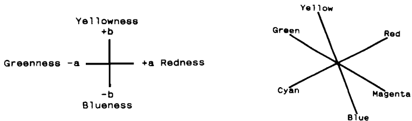
Figure 1. The L, a, b or L*, a*, b* instructions as normally explained, versus plots of perfect colors on the L, a, b diagram. The color terminology for the "a" axis is not precise.
