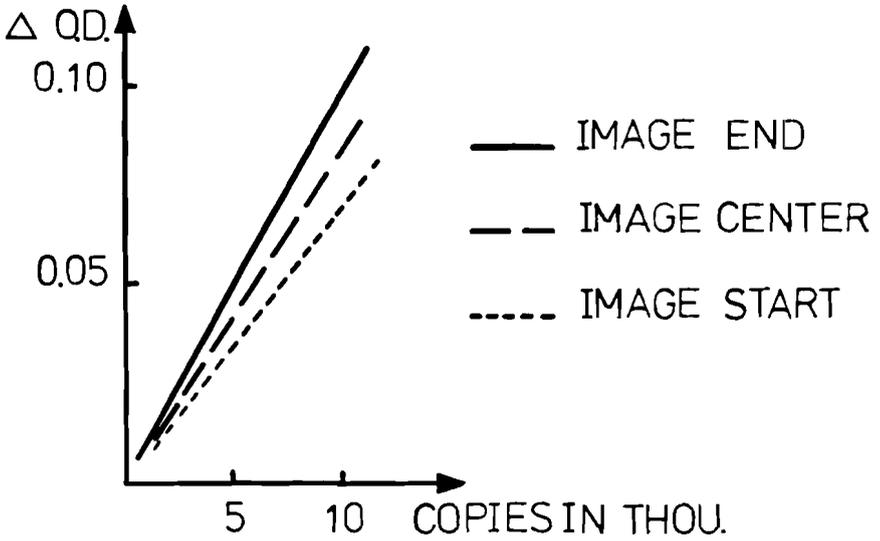
Fig. 10 :  $\Delta$  O.D. of bottom print versus no. of copies for different locations on the plate (second trial, paper C, B1 50 % top on M2 50 % bottom).
