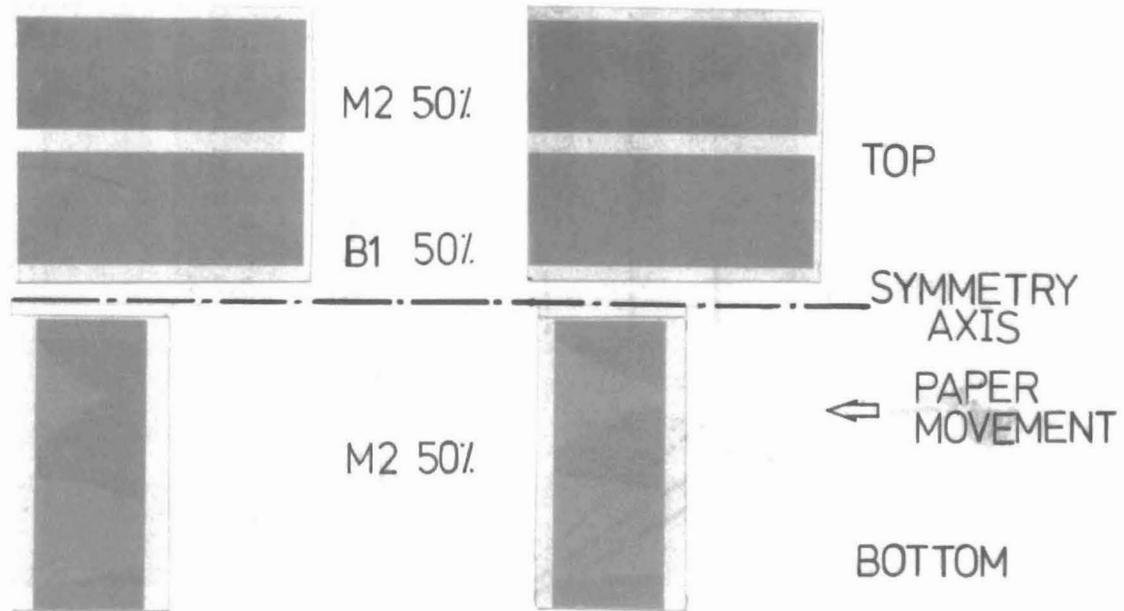
Fig. 11 : Increase in surface covered by ghosting from image start to image end for direct and backtrap ghosting (second trial, paper C).
