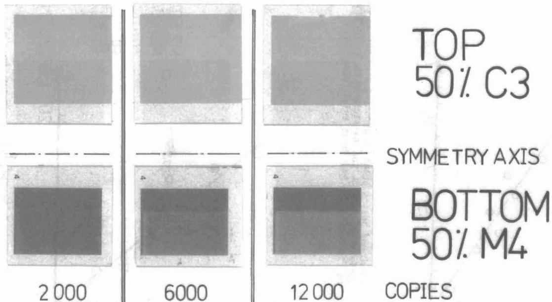
Fig. 7 : Increase in ghosting on the bottom side versus no. of copies, first trial, paper C (Variations in O.D. on the top are due to print through).
