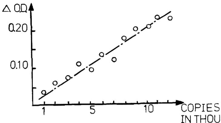
Fig. 8 :  $\Delta$ O.D. of bottom print in ghosting area versus no. of copies for a 50 % top halftone upon a 50 % bottom halftone (C3 upon M4, first trial, paper C).
