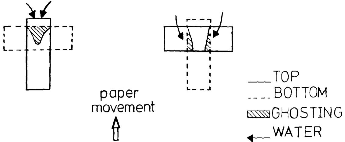
Fig. 16 : Patterns of ghosting caused by different top printing orientations. The solid lines indicate orientation of the top print and dotted lines the orientation of the bottom print. Water flow, indicated by the arrows, is believed to cause ghosting.
