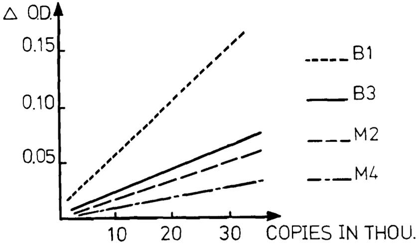
Fig. 12 :  $\Delta$ O.D. from direct ghosting for paper A with the four inks (second trial, 50 % top on 50 % bottom).
