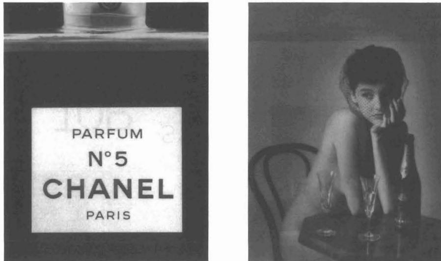
Fig. 1 : An industrial example of mechanical ghosting. The reduction in optical density can be seen in the reversed letters and outside the square in the illustration on the right, corresponding to the white square and the black letters on the left.
