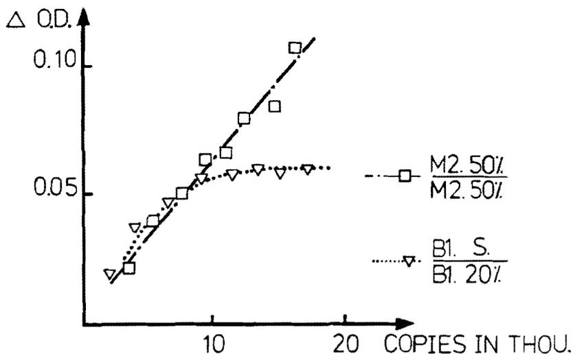
Fig. 9 :  $\Delta$ O.D. of bottom prints versus no. of copies, illustrating a rapid stabilization for a large difference between top and bottom coverage. Stabilization has not yet occurred for the situation where top and bottom coverage is the same (paper C, second trial).
