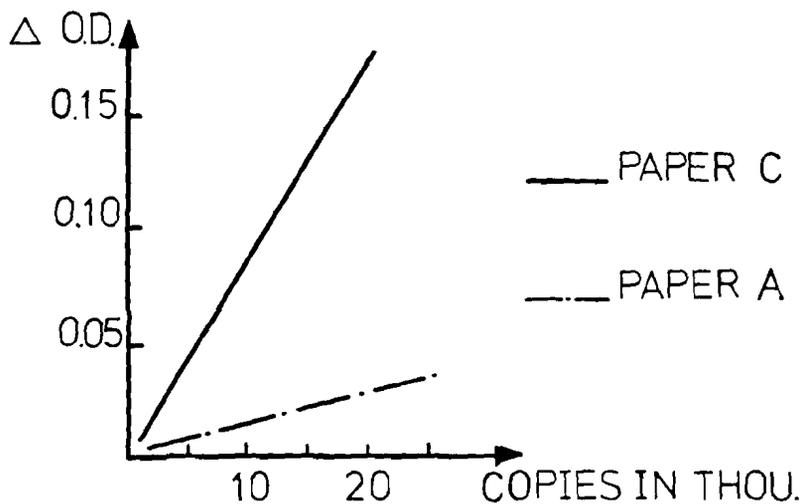
Fig. 14 : Difference in behavior for backtrap ghosting with papers A and C (second trial, B1 50 % top on M2 50 % bottom).
