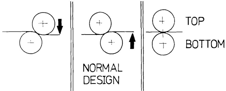
Fig. 6 : Three blanket-to-blanket press designs. The most common appears in the center. Web direction is always from left to right. Location of ghosting is indicated by the arrows.
