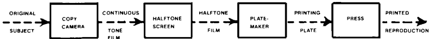
FIGURE 1 Block Diagram Representation of a Simple Photomechanical Printing Process. In this model, blocks represent stages in the process and dashed lines represent stage inputs and outputs.
