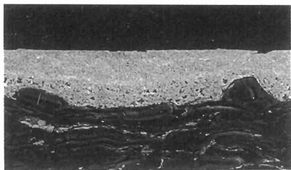
Fig 13a. Cross section of coating with wet pick. This corresponds to the area of Fig 9a at 1000 X
