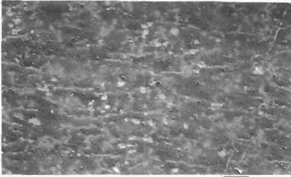
Fig 7a. Complaint sample showing grainy mottle. 100 \mu m at 100 X
