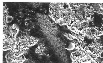
Fig 6b. IGT Wet pick at a higher magnification. | 10 \mu\text{m} at 1000 X
