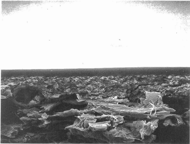
FIG. 19 - ULTRAVIOLET OVERCOATING OF PRINTED BOARD - 1500 X
