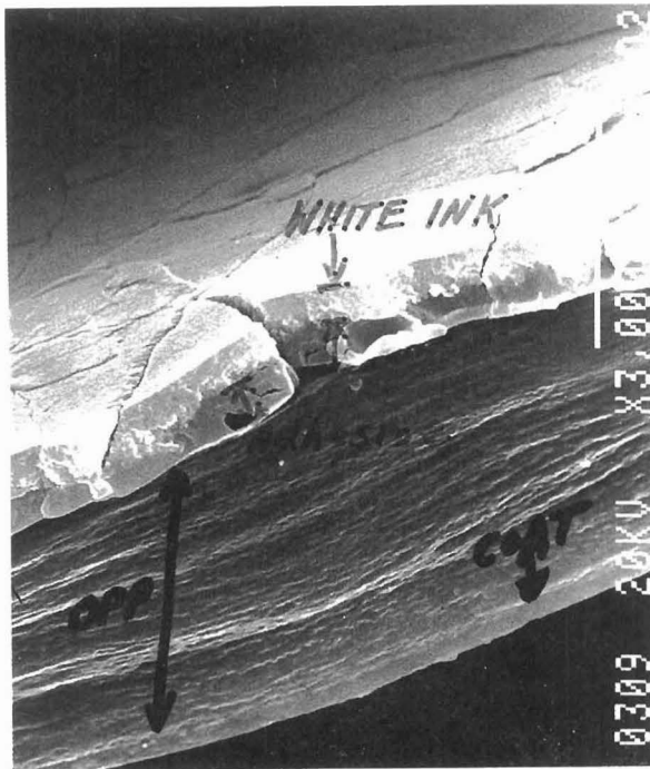
FIG. 24 - WHITE OVER COLORED FLEXO INK ON REVERSE COATED POLYPROPYLENE-3K X
