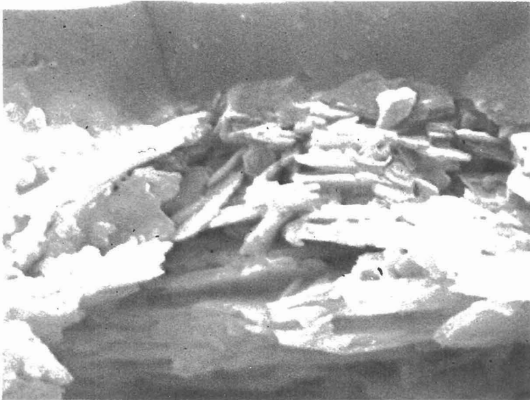
FIG. 12 - PUBLICATION GRAVURE SOLVENT INK ON COATED PAPER - 20K X
