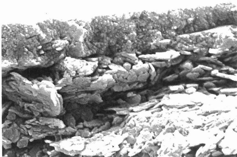
FIG. 20 - WATER BASED PUBLICATION GRAVURE INK ON COATED PAPER - 12K X
