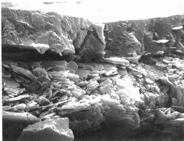
FIG. 21 - SOLVENT BASED PUBLICATION GRAVURE INK ON COATED PAPER - 12K X
