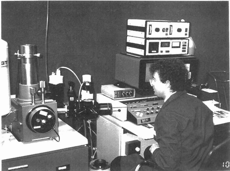
FIG. 4 - SEM EQUIPPED WITH CRYOFRACTURE ATTACHMENT FOR LIQUID SAMPLES
