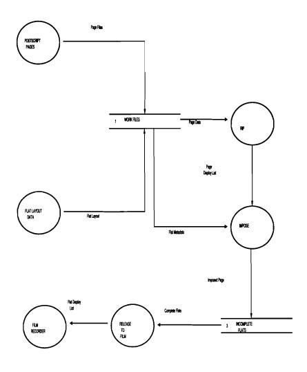
Figure 4 Device dependent imposition.
