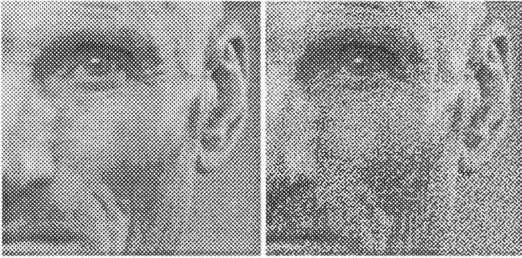
Figure 2. The original image and its stochastic representation as viewed from a distance 254 mm using a resolution of 12 dots/mm.
