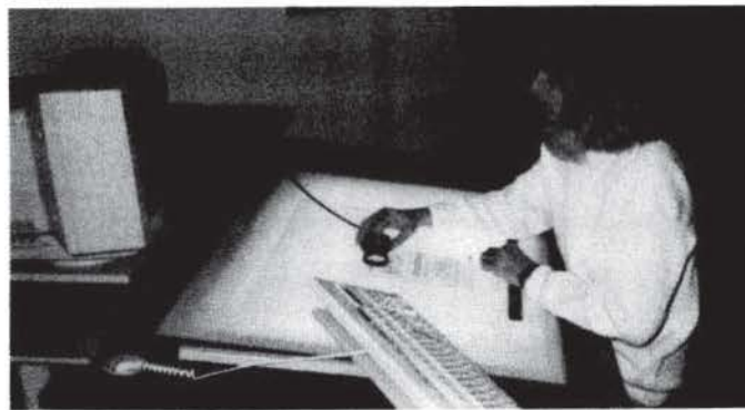
Figure 3. Place one of the mounted foils on register pins of the Job Preparation Station.
