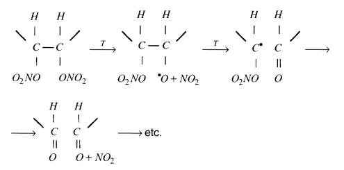
Thus forming dialdehydes then react with the formation of a solid residue having a high thermal stability. That is why the non-printing areas of plates 5 are ink-receptive. Presumably the organic dye ablation occures before the polymer destruction or dye's concentration in the polymer composition is insufficient for its volume-heating-up.
