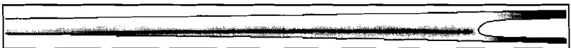
Figure 9: Viscosity differences along the nip ( u_2/u_1=0,33 ; 2H_0=40\mu\text{m} ), (black-17,5 Pa·s; lightgray-12,5 Pa·s= \eta_\infty )
