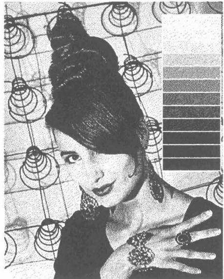
Figure 11. Halftone using Floyd & Steinberg error distribution and 50% randomness applied to the threshold level
